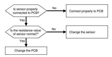
\*\* In case the value is more than  $100k\Omega$  (open) or less than  $100\Omega$  (short), Error occurs
